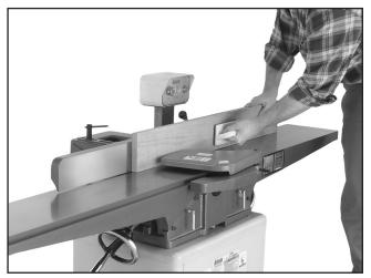
Figure 30. Typical edge jointing operation.
